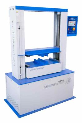
Core Compression Tester Instrument is widely used in the "Paper & Packaging Industry" for determination of crush or compression resistance of paper cores, such as used for winding rolls of plastic film.
